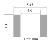
Figure 11. Recommended PCB Pad Size
