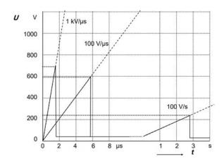
Figure 2. Spark-over Voltage Waveform
