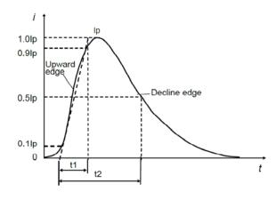
Figure 3. Impulse Discharge Current Waveform
