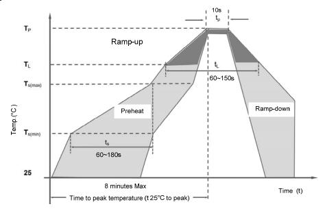
Figure 9. Reflow Soldering
