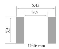
Figure 11. Recommended PCB Pad Size
