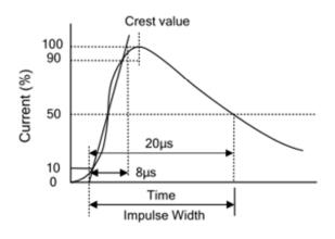
Figure 3. Impulse Discharge Current Waveform
