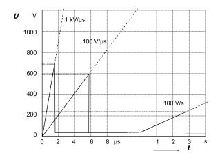
Figure 2. Spark-over Voltage Waveform
