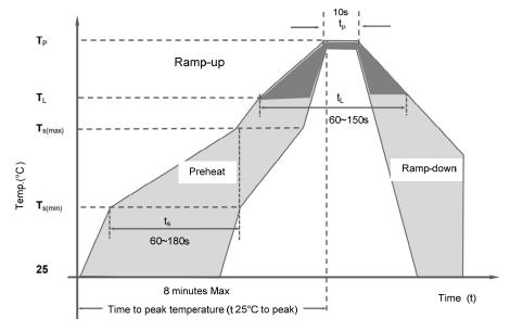
Figure 9. Reflow Soldering
