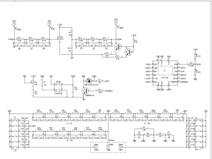
Figure 7. Schematic of TEC Controller Evaluation Board TEC14MEV1.0
