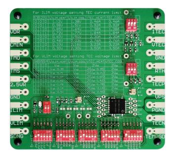
Figure 1. The Physical Photo of TEC14MEV1.0
