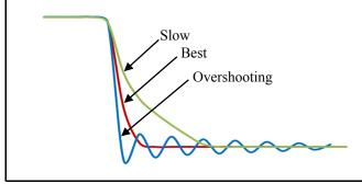
Figure 9. Fall Waveforms of VTEC
