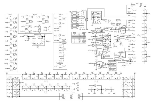
Figure 10. Schematic of TEC28V15AEV2
