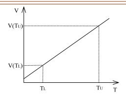
Figure 22. Temperature sensor IC characteristics
