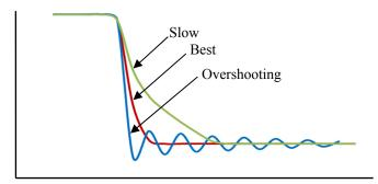
Figure 12. Fall Waveforms of IDR
