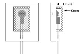
Figure 3. Using an Insulation Cover to Improve Accuracy
