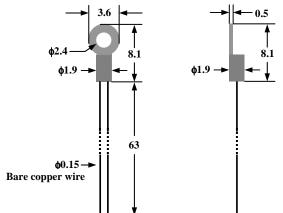
Figure 2. The Front and Side Views of ATH100KL2A
