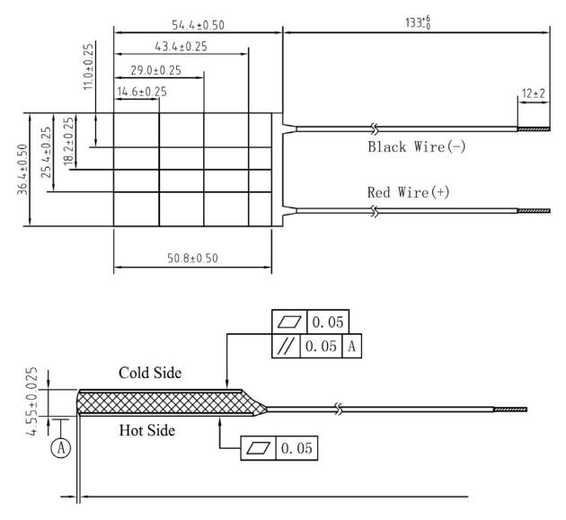
The head of the RTV sealing shall be 0.5 maximum out of the module's edge, except for where near the soldered ends of the lead wire.
